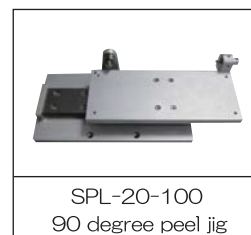
SPL-20-100 90 degree peel jig Max. load 20 N Mounting screws M5×4 Moving distance 100mm
